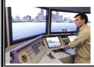
Technically called a Full Mission Bridge Simulator, it has highly detailed virtual reality seascape and landscape features, including correctly positioned buildings, ship facilities, and even TAMUG campus structures on their sites in the Galveston ship channel. It's the operator's job to guide his ship through the channel safely and efficiently as he watches the video screens.
